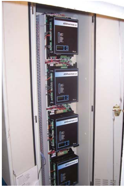
The static drives on a Marion shovel had become unreliable and obsolete (left), they were replaced with Avtron Firing Modules (right) and machine availability improved dramatically.
