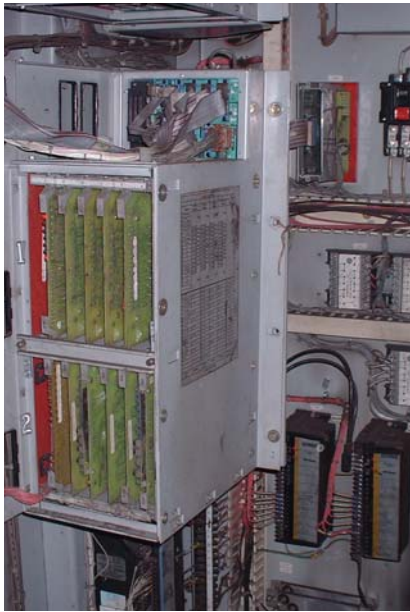
The static drives on a Marion shovel had become unreliable and obsolete (left), they were replaced with Avtron Firing Modules (right) and machine availability improved dramatically.
