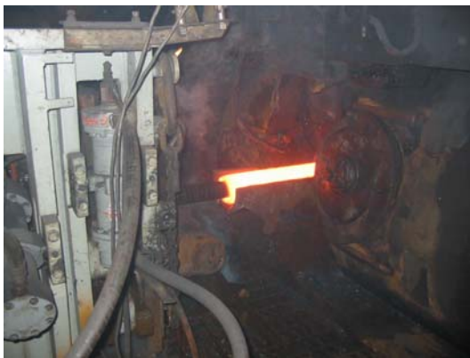
Figure 5 – Tube being Pierced on #5 Tube Mill
